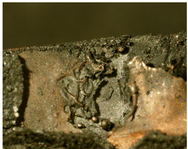
Fig. 4. Ground zero arc damage on the copper foil substrate on a torn side fold near the bottom corner of cell #5.
