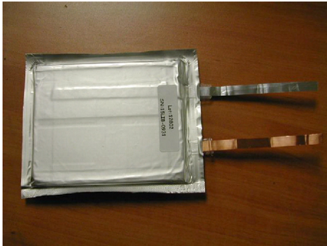
Fig. 1. One of the five cells that make up a cell module.
